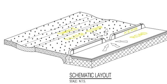
TYPICAL ROADSIDE LATERAL KERB INLET (NON-CONTINUOUS KERB)
